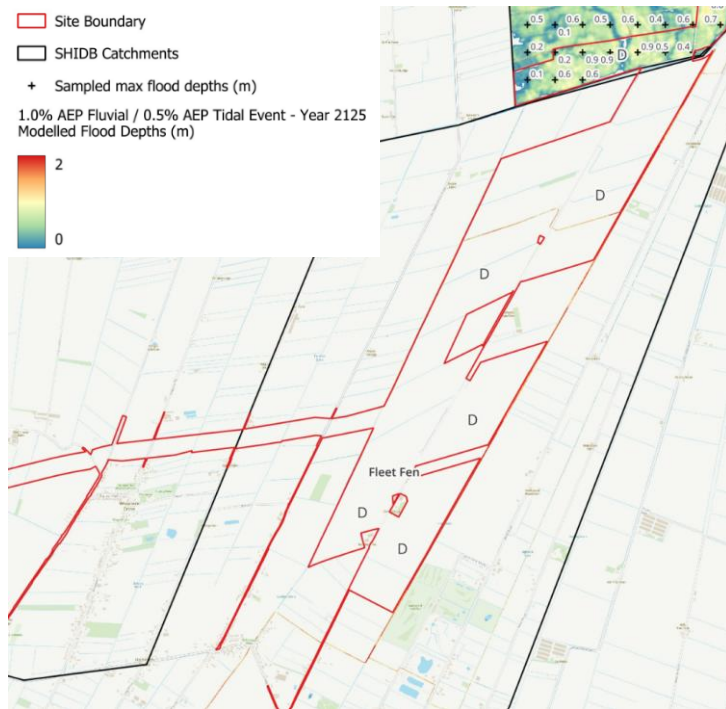
Plate 5-8: 1% AEP plus 13% climate change Pump On Scenario flood extent in the Fleet Fen Catchment
